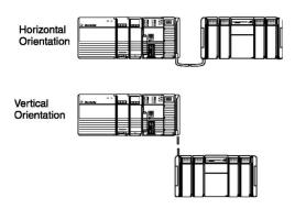
How you orient I/O banks determines which expansion cables you need to connect the I/O banks.
